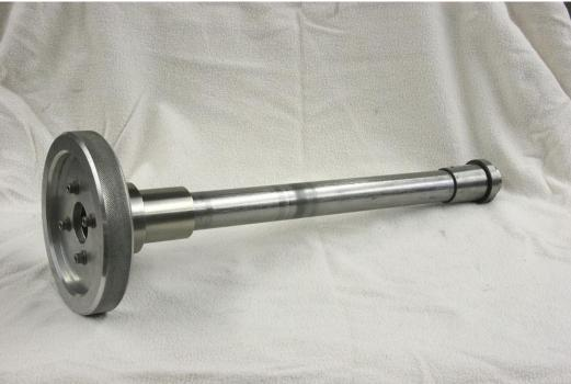
Set up is fast and easy. The 5C collet to 5 Morse adapter is placed in the spindle nose by hand, the closer tube inserted into the spindle bore, and the collet of choice threaded into the brazed in internally threaded steel insert in the end of the 4140 tube. A twist of the handle, and you are ready to turn your part.
