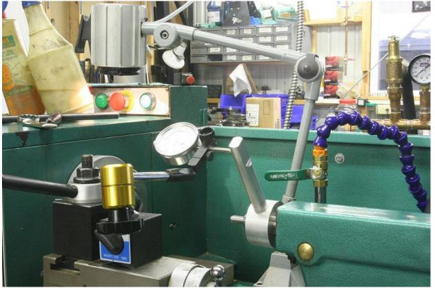
This setup is used when chambering, and allows for a repeatable and precise indication of how far the reamer has advanced. The dial indicator is fixed via a magnetic base to the locked cross slide, and bears on a shop made arm attached to the tailstock spindle.
