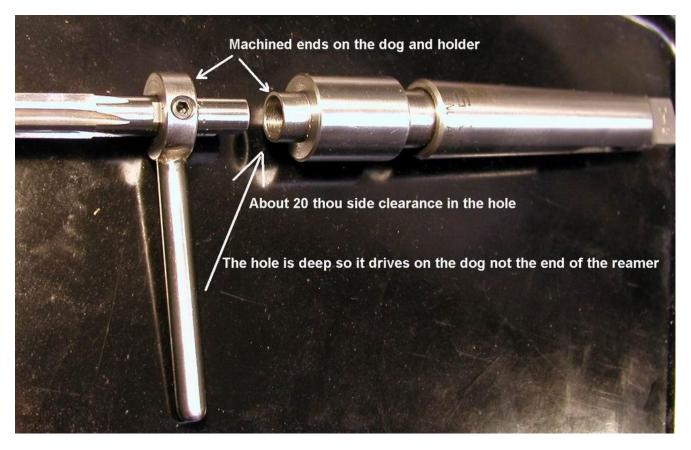
Actually, the credit doesn't go to me for driving the **reamer** like that. I just made it, used it and put it in the barreling article on my web site. Dave Tooley told me about it and is where the credit goes. I use a Sinclair case **holder** to hold the **reamer** and Albrecht chuck to hold the tube that pushes the **reamer**. The Bald Eagle **floating reamer holder** works similarly
