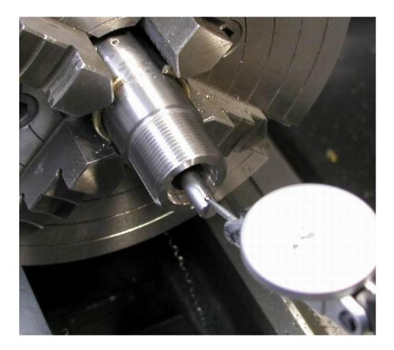
These runout posts are very interesting reading. There seems to be two perspectives on setting up the barrel for cambering that include indicating the muzzle and breech end to run with each other, somewhat the same as between centers, and the other one being setting the chamber end bore straight without regard to the muzzle runout. Does anyone change their method depending on the amount of bore curve found in the barrel?
