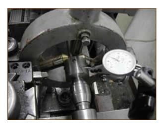
Adjusting steady rest to true bolt face. The dial indicator is to check that the bolt body doesn't move when steady rest points are adjusted.
