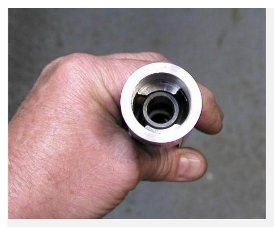
Here is a different action after very lightly lapping the lugs with 600 grit to confirm the fit. Both lugs have good contact. The only reason the front of the lugs and the nose of the bolt are machined is for a more accurate measurement when fitting the barrel.
