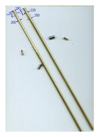
You'll notice that there is a step in the smaller rod I will probably turn it down to .200 the rest of the way down the rod until there is only about 1" left unturned so the rod isn't trying to flex in to places. James
