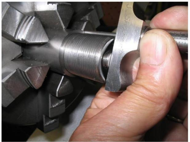
It is almost impossible to get an accurate headspace reading since the micrometer will cock over and give a false reading. Instead, make a measuring collar and do this-
