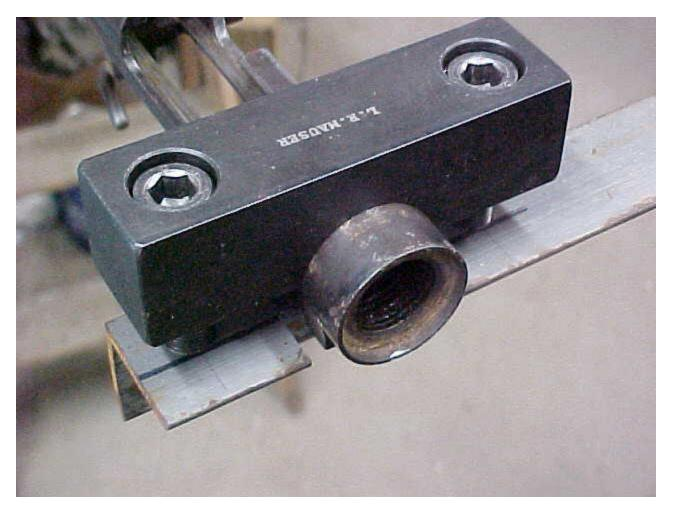
This shows the "economy" handle, just a piece of bedrail, with two holes and a notch. This one is about 3 feet long with the action at the end. If your bench/shop will stand the extra length, use a four foot piece and but the action in the middle. Then two of you can use it, one on each end.
