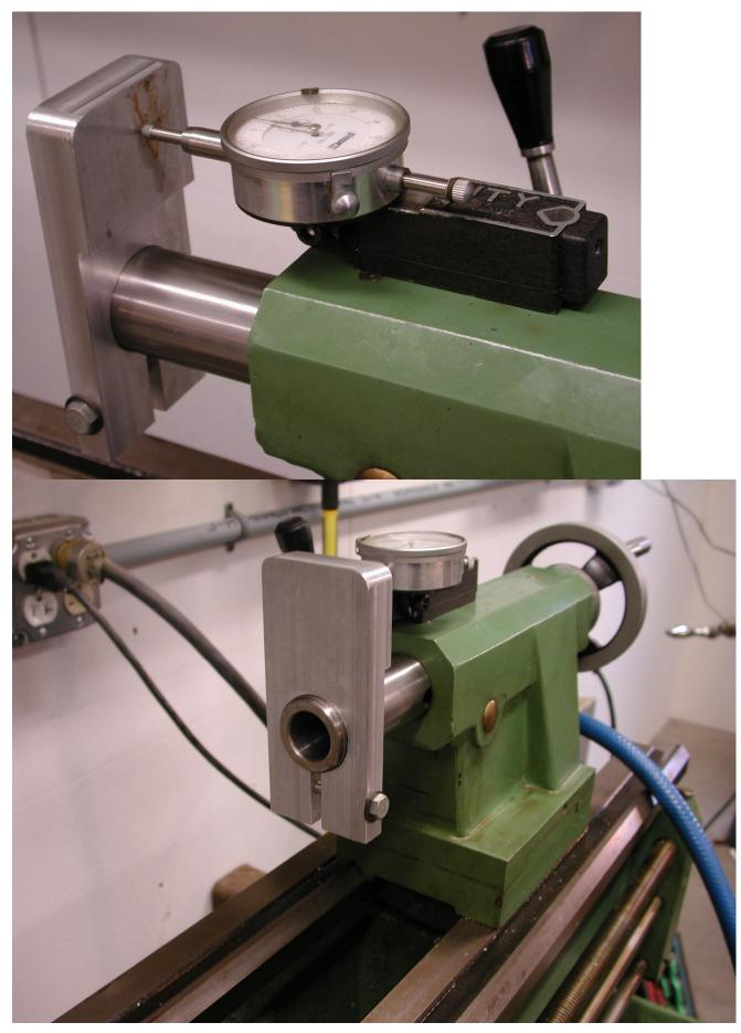
This is the "Cat Head" or Spider I made to go on the back end of the spindle.
