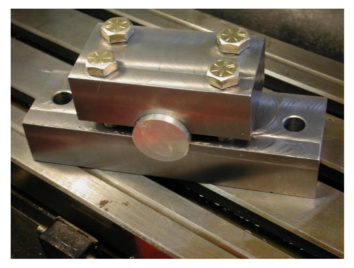
The mounting holes were drilled 9/32" to use  $\frac{1}{2}$ " mounting bolts. The base piece is 8" long.
