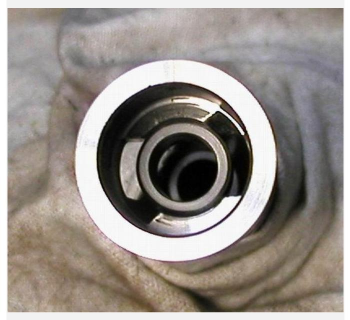
Here is one picture of the action with the front bushing still in after re threading and facing.
