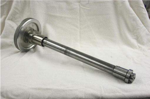
This view shows the unit assembled. The outboard end rides on a collar that floats over the spindle OD, and the axial thrust is taken up with a Torrington bearing built into the collar.
