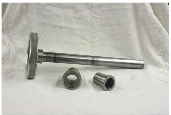
This is a shop made 5C handwheel type collet closer. A factory unit was not available from Grizzly for the G9036 lathe, so I made one using some stainless, aluminum, and 4140 tube stock. The only part that was not shop made was the precision ground 5C collet adapter that fit in the headstock spindle
