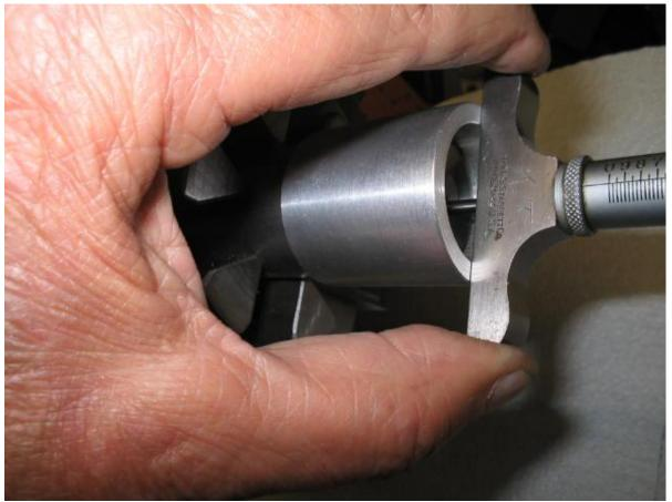
Using a collar as shown is the most accurate method since the micrometer makes rigid contact on both sides of the collar and cannot cock over.
