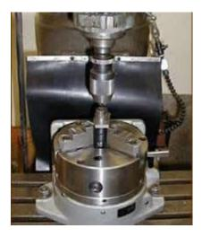
nreads. Drilling receiver to pin Holland recoil lug.
