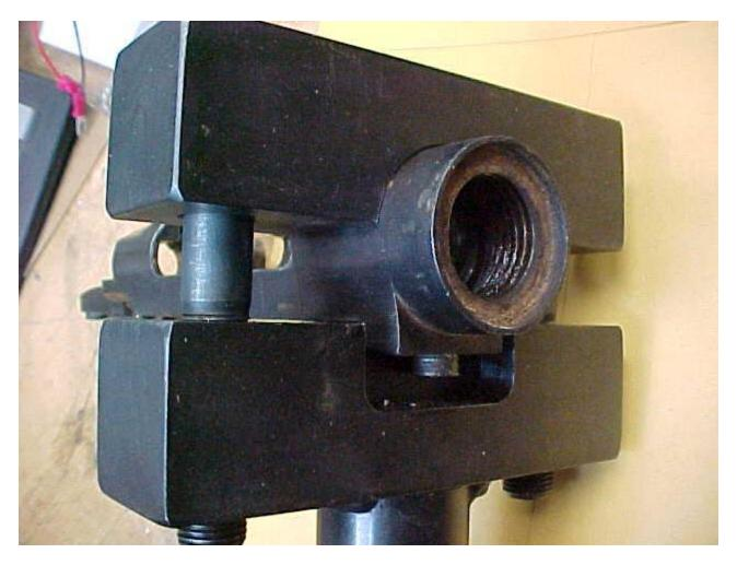
This shows the <u>Brownells</u> action wrench in action. If the action was blued, an aluminum shim could be wrapped around the top half of the action. But, take note of the cutout portion of the handle that allows for the recoil lug. If not for this cutout, the wrench could be made form a solid bar, with two holes, tapped or not, for the bolts.
