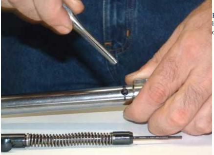
By pushing the bolt head in towards the bolt it should be possible to push the pin out of the bolt. Here are the parts layed out along withthe new bolt head. Note the spring washer between the baffle and the bolt body. It provides spring tension on the bolt head to retain the bolt head pin when the striker assembly is removed.
