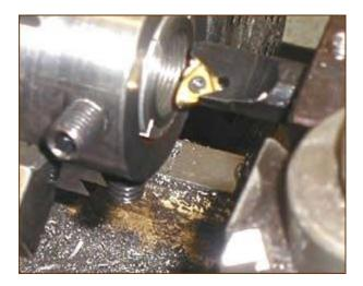
Single point re-cutting the receiver threads.
