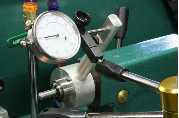
In this view, you can see how the indicator will stay in position even after the tailstock is removed and returned to place. This allows for easy and fast measuring of the headspace dimension, and allows a precise indication of how much the reamer advances during cutting. Achieving less than 0.001 inch precision in final chamber headspace is routine and very easy with this setup.
