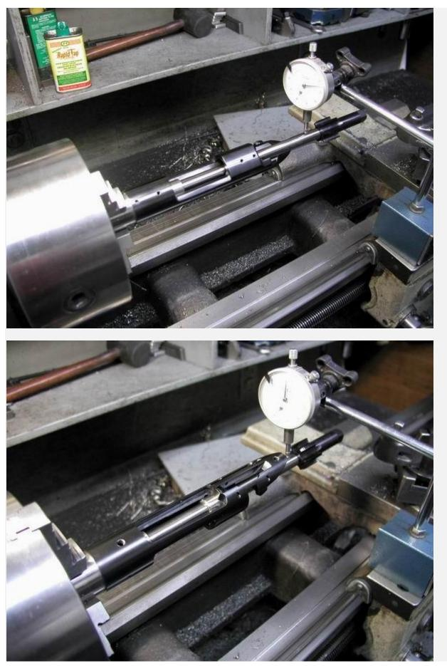
This is a picture showing although the front and one lug recess are faced true it still needs more facing as the other lug recess is untouched...
